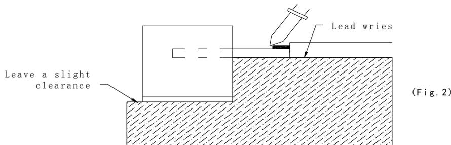
Regarding solution in the tinning oven for product-tinning, compound sub-solution made of tin & copper and silver is proposed with the temperature of Celsius 260. The proportion of the alloyed solution is tin 95.5: copper 3.5: silver 0.5 by percentage. The time of tinning is constantly 3 seconds.
