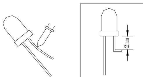
2) Forming lead should be carried out prior to soldering and never during or after soldering.
