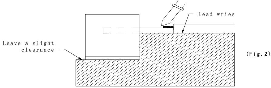
Regarding tinning the leads, compound made of tin ,copper and sliver is proposed with the temperature of 260°C. The proportion of the alloyed solution is 95.5% tin, 3.5 % copper, 0.5% silver. The time of tinning is 3 seconds.
