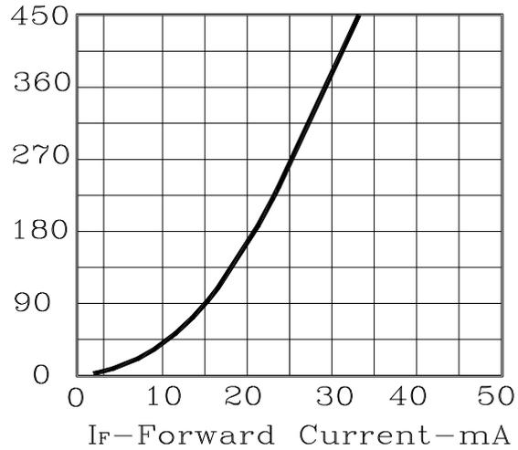
■ Duty Ratio vs. Allowable Forward Current
