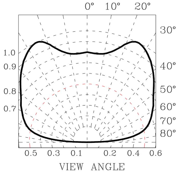
5.0 mm DIA CYLINDRICAL LED LAMP
