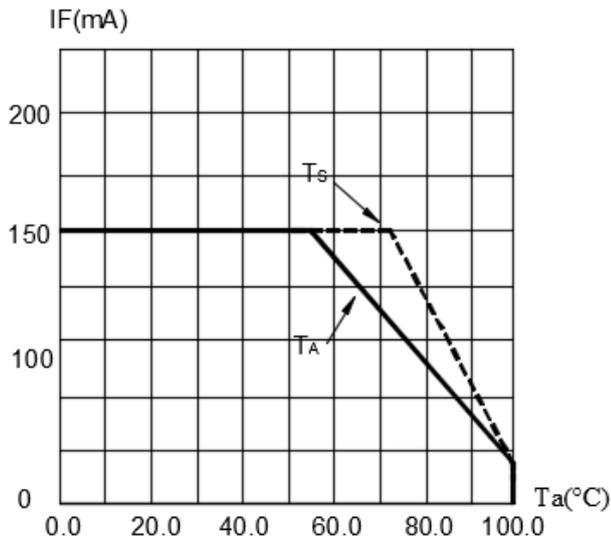
FIG.2 MAXIMUM FORWARD DC CURRENT VS AMBIENT TEMPERATURE ( $T_{jmax}=120\text{ }^{\circ}\text{C}$ )
