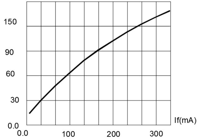
FIG.3 RELATIVE LUMINOUS INTENSITY VS. FORWARD CURRENT
