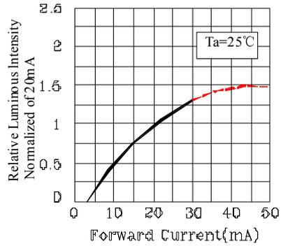
Fig. 2 Relative Luminous Intensity vs. Forward Current
