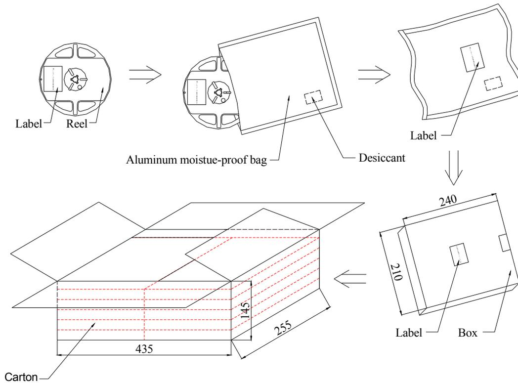
Notes : One reel in a bag, one bag in a inner box, ten inner boxes in a carton. Unit : mm.
