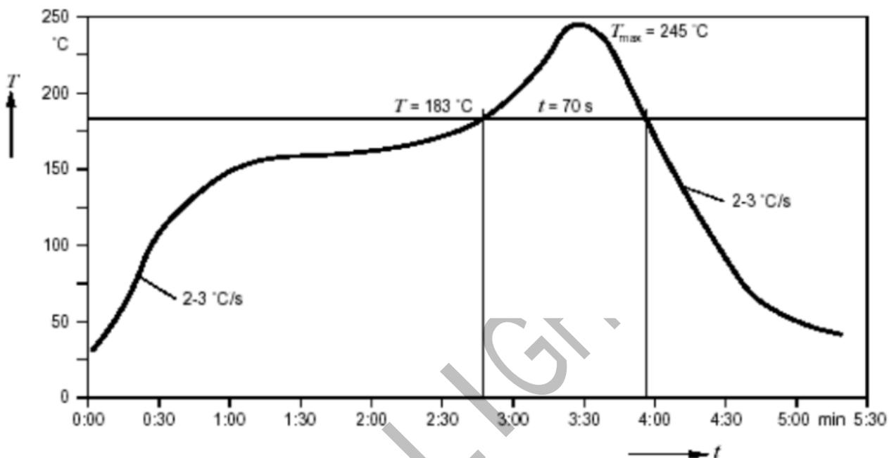
● Suggest Pb-Free IR Reflow Soldering Profile Condition:
