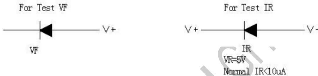
3. If the forward voltage VF is too high or the reverse voltage VR is too high, the LED will be damaged.
