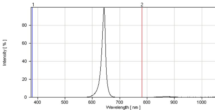
Fig.1 Red Relative Intensity vs. Wavelength
