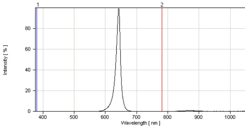
Fig.1 Red Relative Intensity vs. Wavelength
