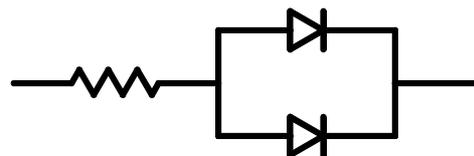
(B)The difference of brightness between LED`s could be found due to the Vf-If characteristics of LED.
