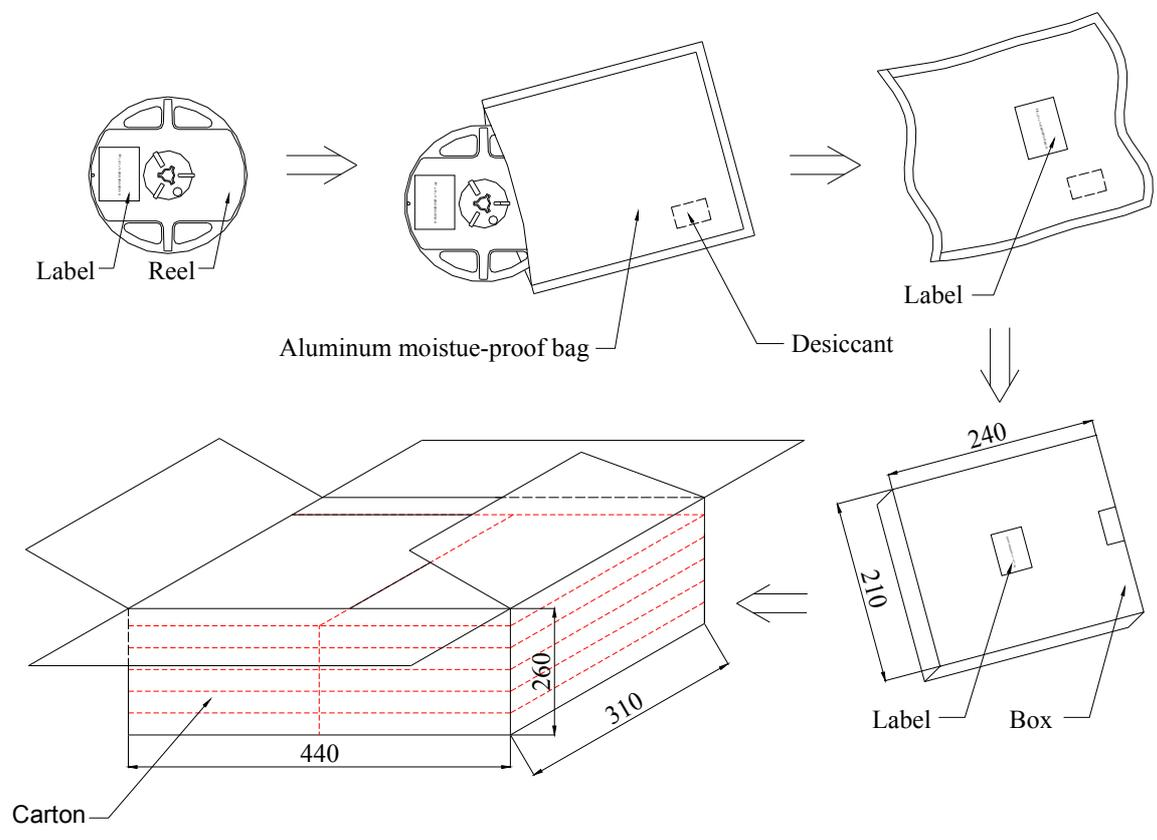
Notes : One reel in a bag, six bag in a inner box, six inner boxes in a carton. Unit : mm.
