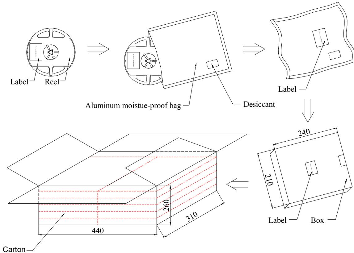
Notes : One reel in a bag, six bag in a inner box, six inner boxes in a carton. Unit : mm.
