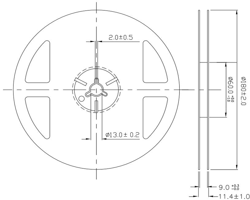
Note: Tolerances unless mentioned  $\pm 0.1$ mm. Unit = mm
