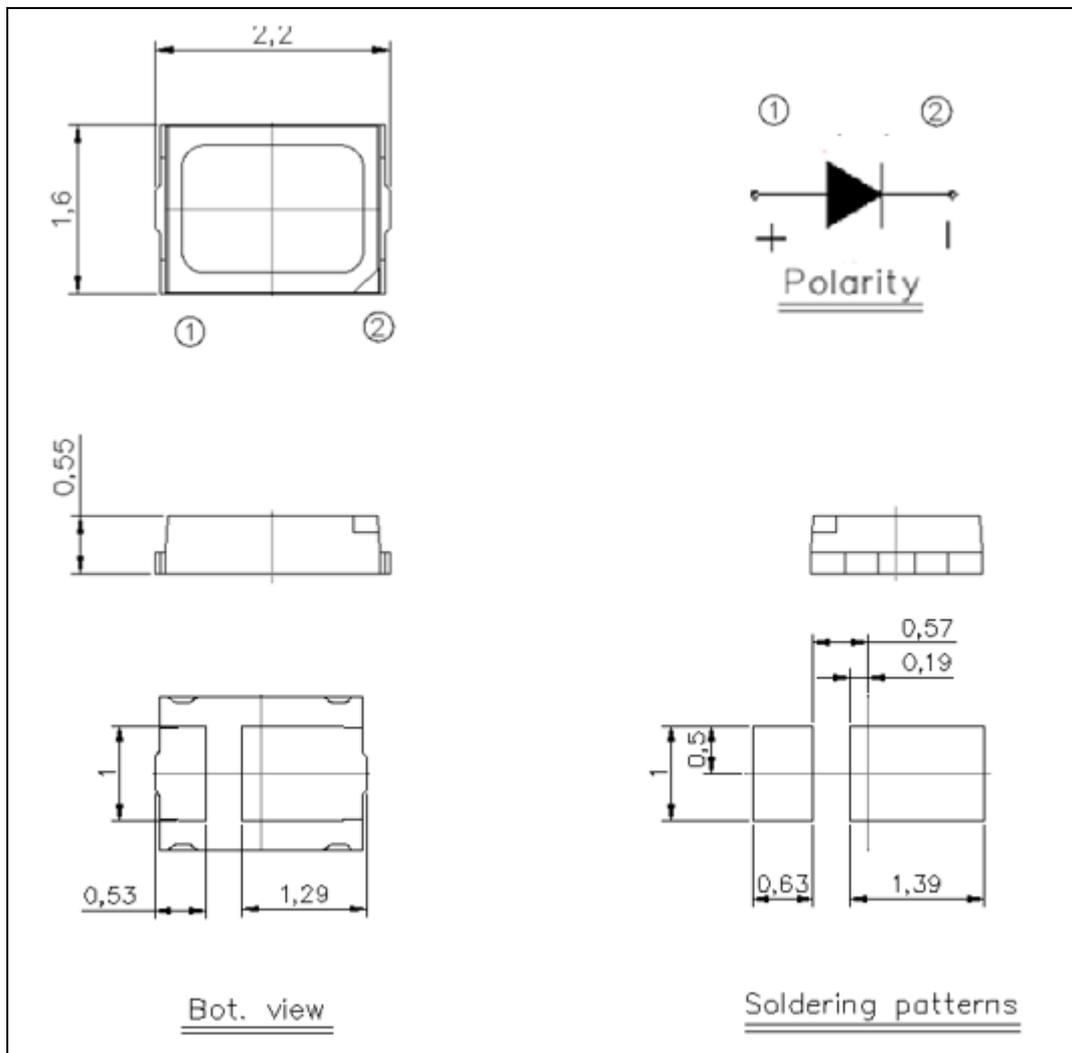
Note: Tolerances unless dimension are  $\pm 0.1$ mm, unit = mm.
